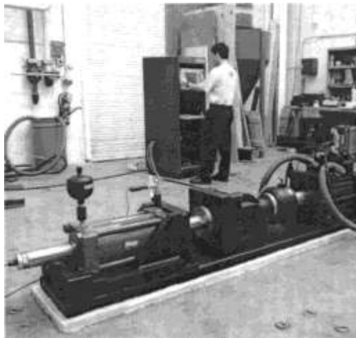
Fig. 6. Experimental setup of the large-scale 20-t MR fluid damper
