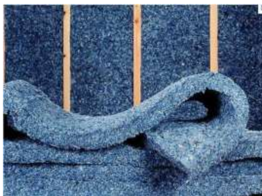
Figure 15: Thermal insulation prepared from denim
