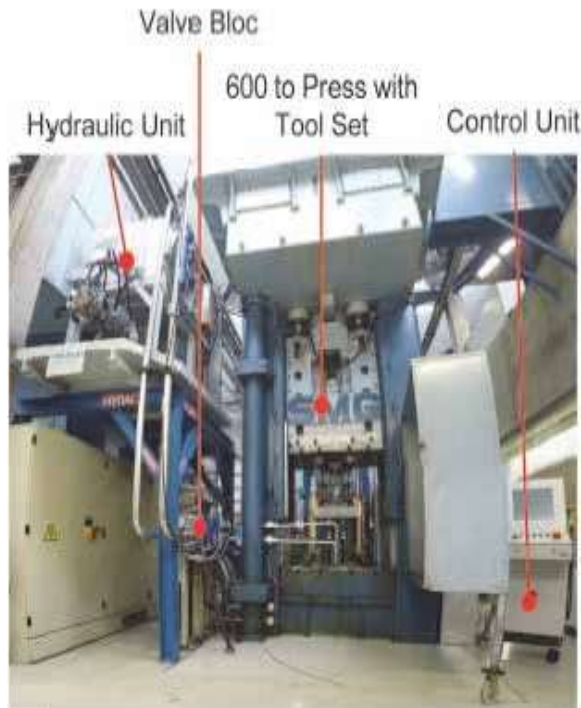
Fig.5. Hydraulic unit with valve bloc, hydraulic press with tool set and control unit
