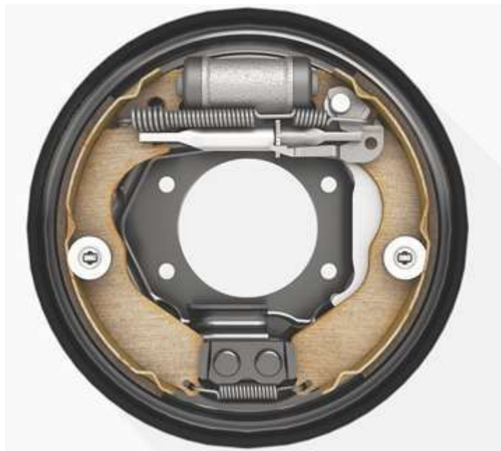
Figure 2: The Brake Applied Load by the Operator on the Pedal Shifted to the Final Brakes Disc or Drum Rotor is known as a mechanical drum brake[3].
