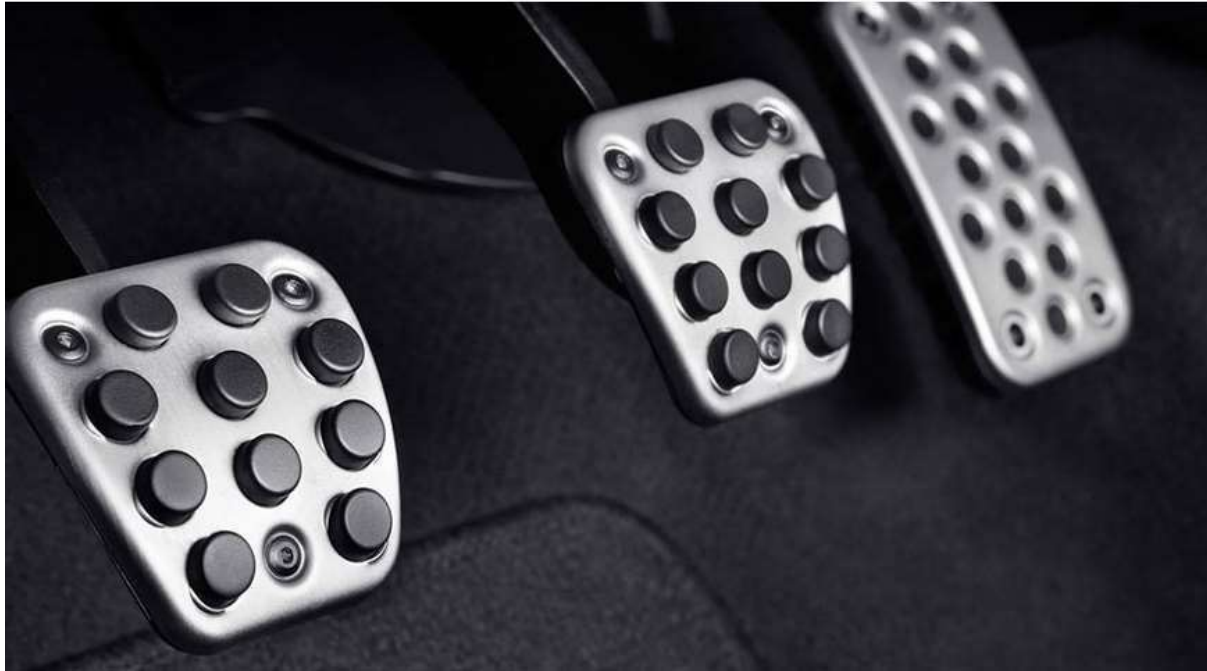
Figure 6: The Brake Form is a Foot Brake in which the Driver uses his foot to push the Brake Pedal mounted within the Cockpit or at the Foot of the Vehicle.
