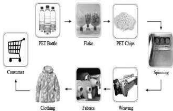
Figure 2. Flowchart showing recycling of PET bottles in to fibers, yarn into fabric
