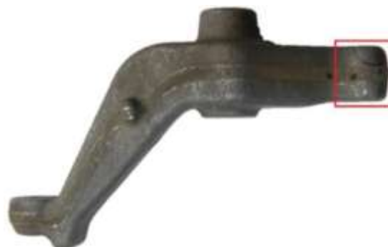
Fig. 3. Defects in lever forging: lap in lever foot
