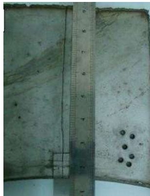
Fig. 14. Crack position and depth in the forging plate.
