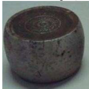
Fig. 8. Upsetting results under different reductions.
