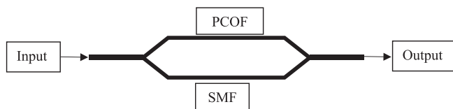
Fig. 5. Proposed optical modulator consisting of a Mach-Zehnder Interferometer (MZI) with one arm of simple single mode fiber (SMF) and the other of a PCOF.
