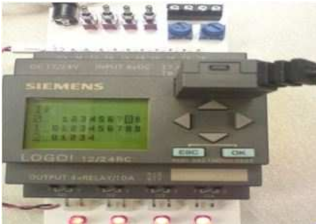
Figure 12. All Gates are open when the radiation level exceeds PLC.
